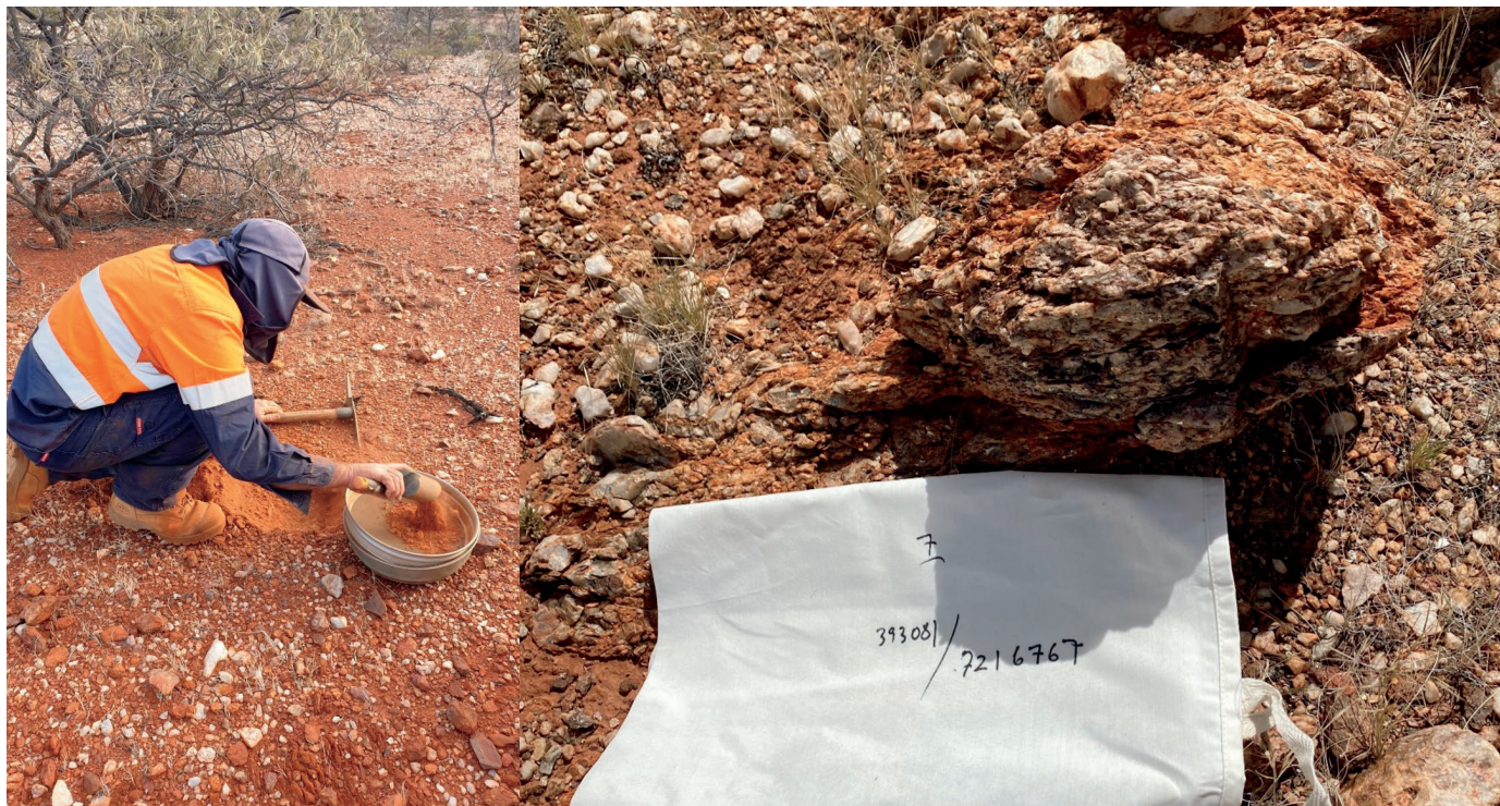
Figure 2 Left - Field Crew Sampling in the Gascoyne. Right - Sample GCRK007, collected from 393081mE/7216768mN (GDA94 z50) - outcropping, 10m wide, plagioclase-quartz-muscovite pegmatite with anomalous LCT signatures (6ppm Ta 2 O 3 , 40ppm SnO 2 & 729 Rb 2 O ppm - refer to Leeuwin IPO prospectus on 28/03/2023 for further information).
