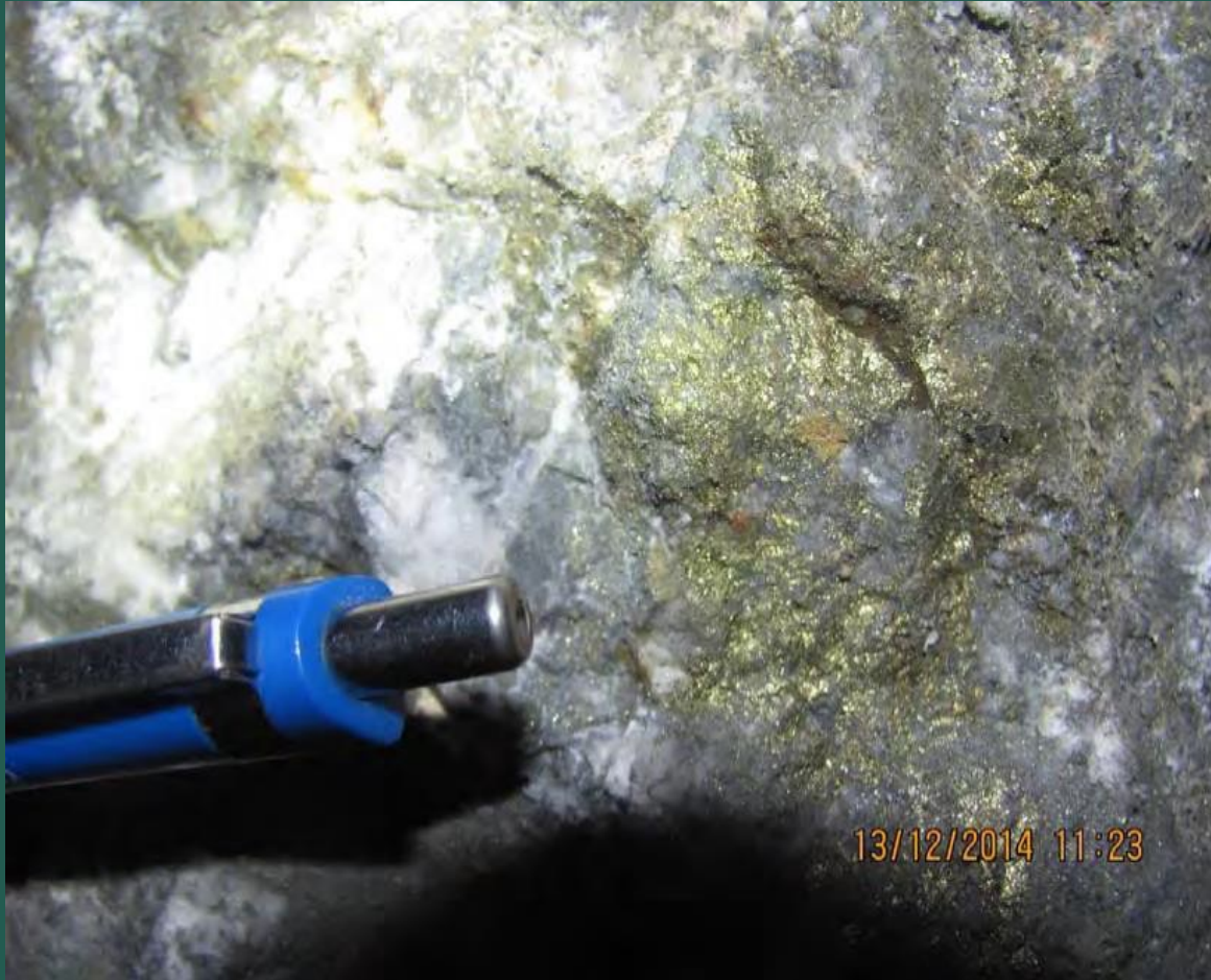
Body 1, in the first cross-cut. Visible chalcopyrite-bornite mineralisation
