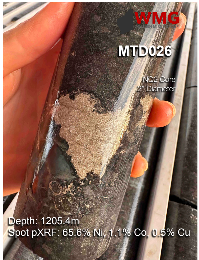
Figure 1: Photos showing examples of visible disseminated sulphides in hole MTD026 with disseminated sulphide forming interstitial blebs between olivine grains Note: core is NQ2 being 2 inches or 50mm diameter
