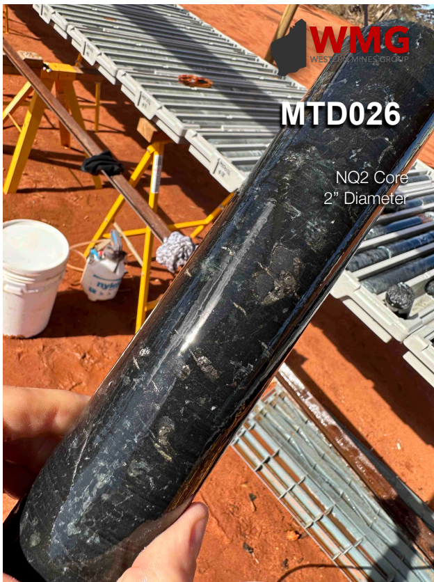
Figure 1: Photos showing examples of visible disseminated sulphides in hole MTD026 with disseminated sulphide forming interstitial blebs between olivine grains Note: core is NQ2 being 2 inches or 50mm diameter
