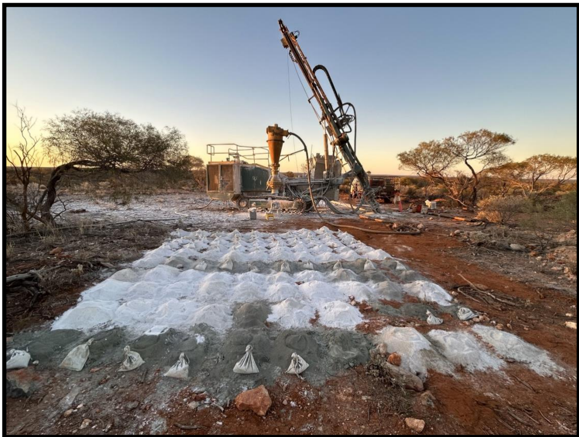
Figure 1: RC drilling at Mt Edon (hole MD23- 07) indicate thick zones (white samples), view to west
