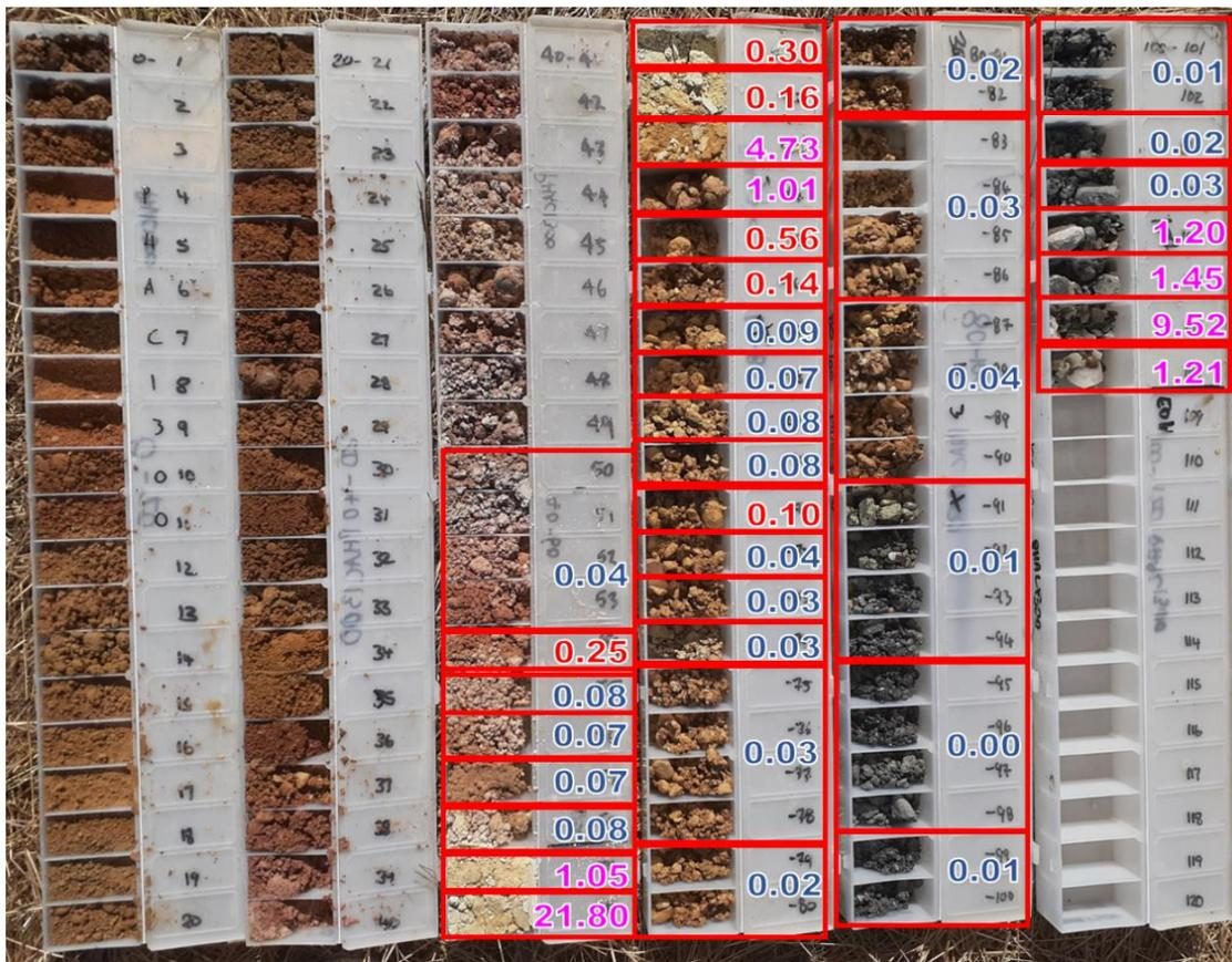
Figure 3 Chip tray photo of hole PHAC1300 showing the high-grade zones (g/t Au) in the saprolite, and in primary mineralisation at the base of the hole
