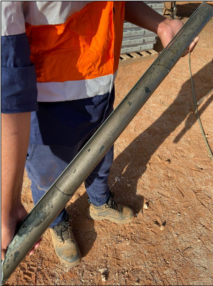
Figure 1: Section of massive nickel sulphide intersected in TED41. See text for further details.
