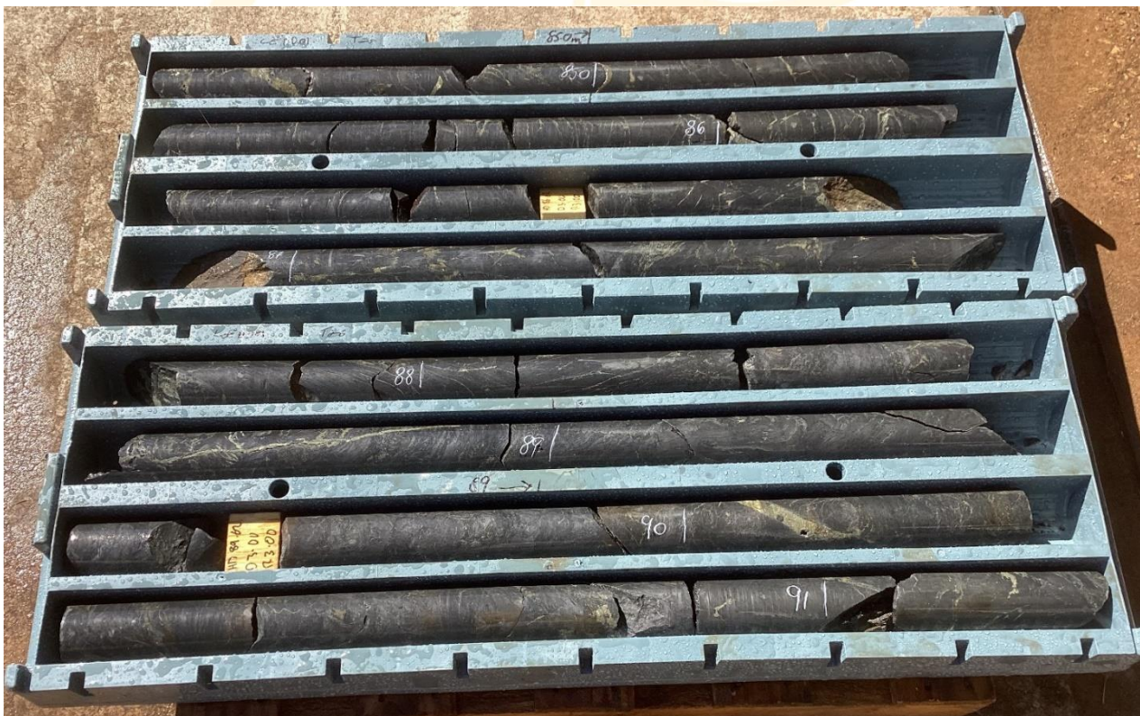
Figure 2: Graphitic Schist LEDD_01 84.5m – 91.3m
