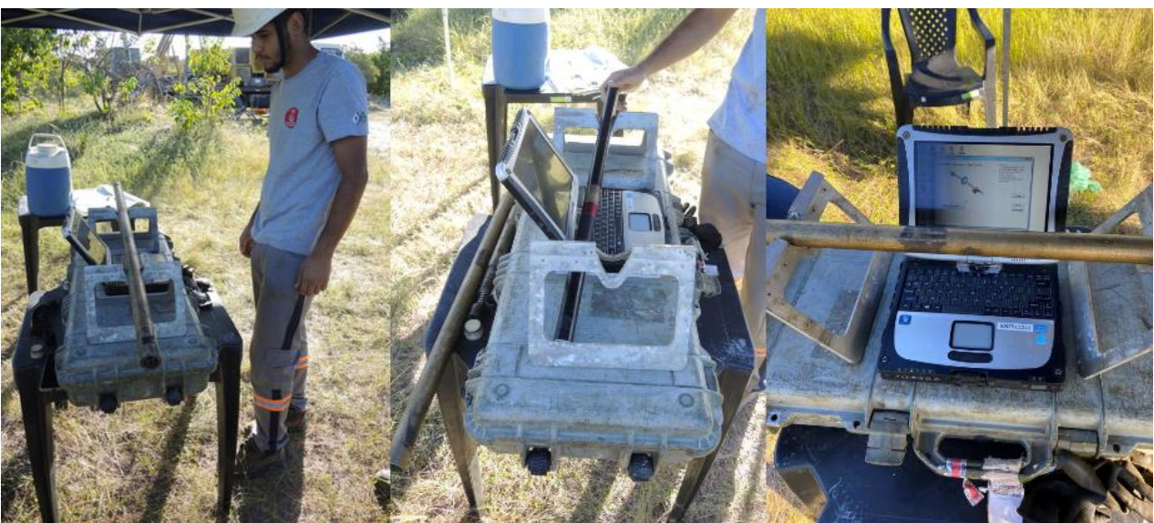
Photo 7 - Downhole survey: downloading hole profile data for viewing on notebook.
