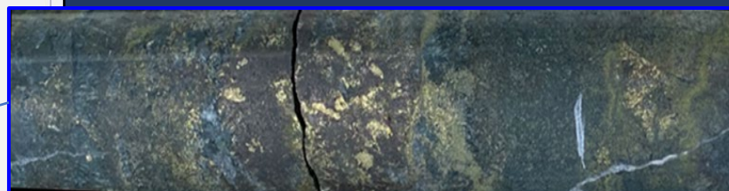
TOP – KIORCDD008 at 197.1m – massive garnet-magnetite-chlorite skarn with chalcopyrite blebs and disseminations on magnetite. BOTTOM - KIORCDD008 at 209.6m – banded magnetite-chlorite skarn with chalcopyrite blebs and disseminations on magnetite.
