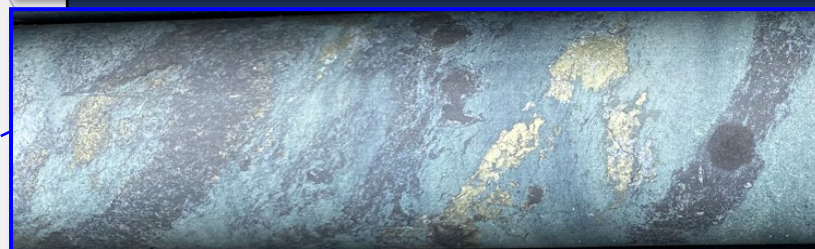
TOP – KIORCDD008 at 197.1m – massive garnet-magnetite-chlorite skarn with chalcopyrite blebs and disseminations on magnetite. BOTTOM - KIORCDD008 at 209.6m – banded magnetite-chlorite skarn with chalcopyrite blebs and disseminations on magnetite.
