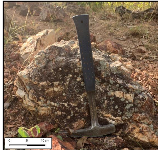
Figure 2. Boulder float showing an example of crustiform quartz veining with pyritic selvages at Molongle.
