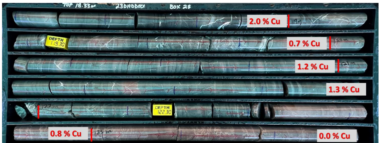
Figure 9: Drill core from 23DHDD001 showing bedded siltstone units with brittle fractures and Quartz-Carbonate veining with chalcopyrite and chalcocite mineralisation from 118-123m.
