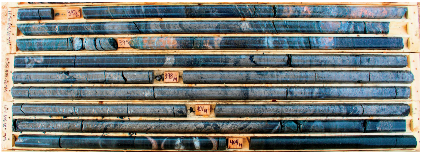
Figure 1: 10.5m of massive to semi-massive nickeliferous sulphides from 392.2m in WL23-368.
