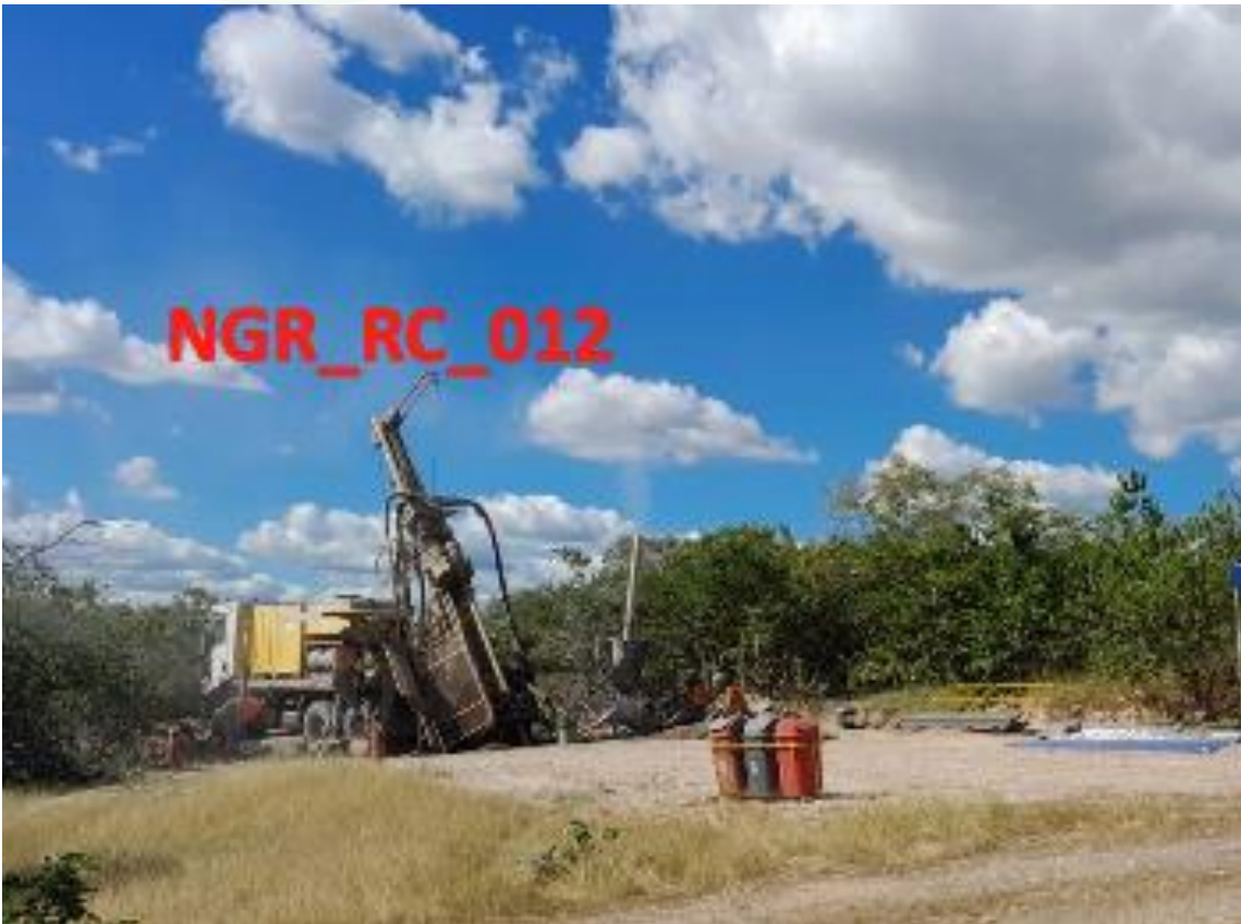
Photo 5 – Inclined RC Hole NGR RC-12 in progress
