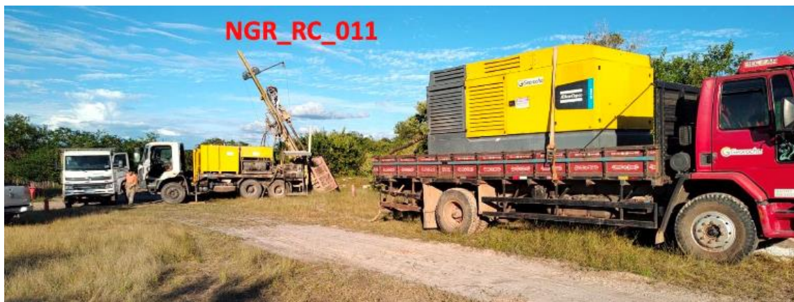
Photo 1 – Drill rig advancing inclined Hole RC-011
