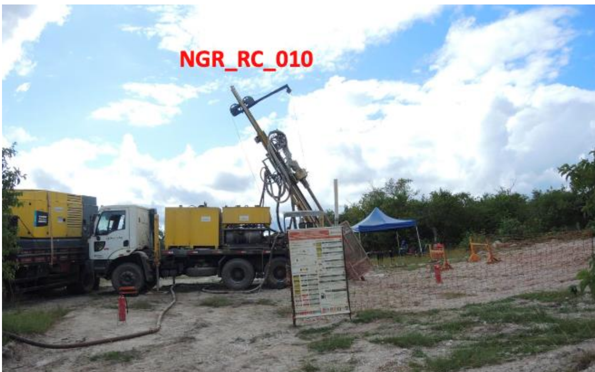
Photo 4 – Inclined RC Hole NGR RC-10 in progress
