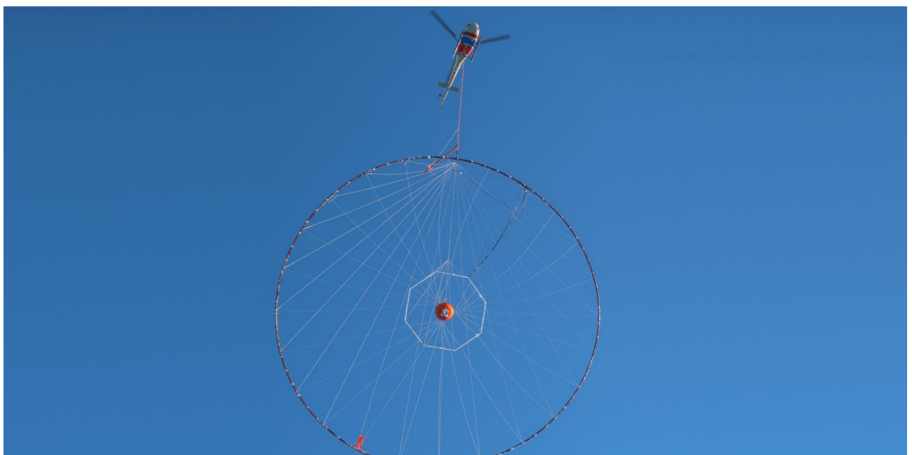
Figure 3: The TargetEM loop under testing
