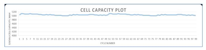
Cycle Life of Volt Natural Graphite Anode in 32650 Lithium Ion Battery
