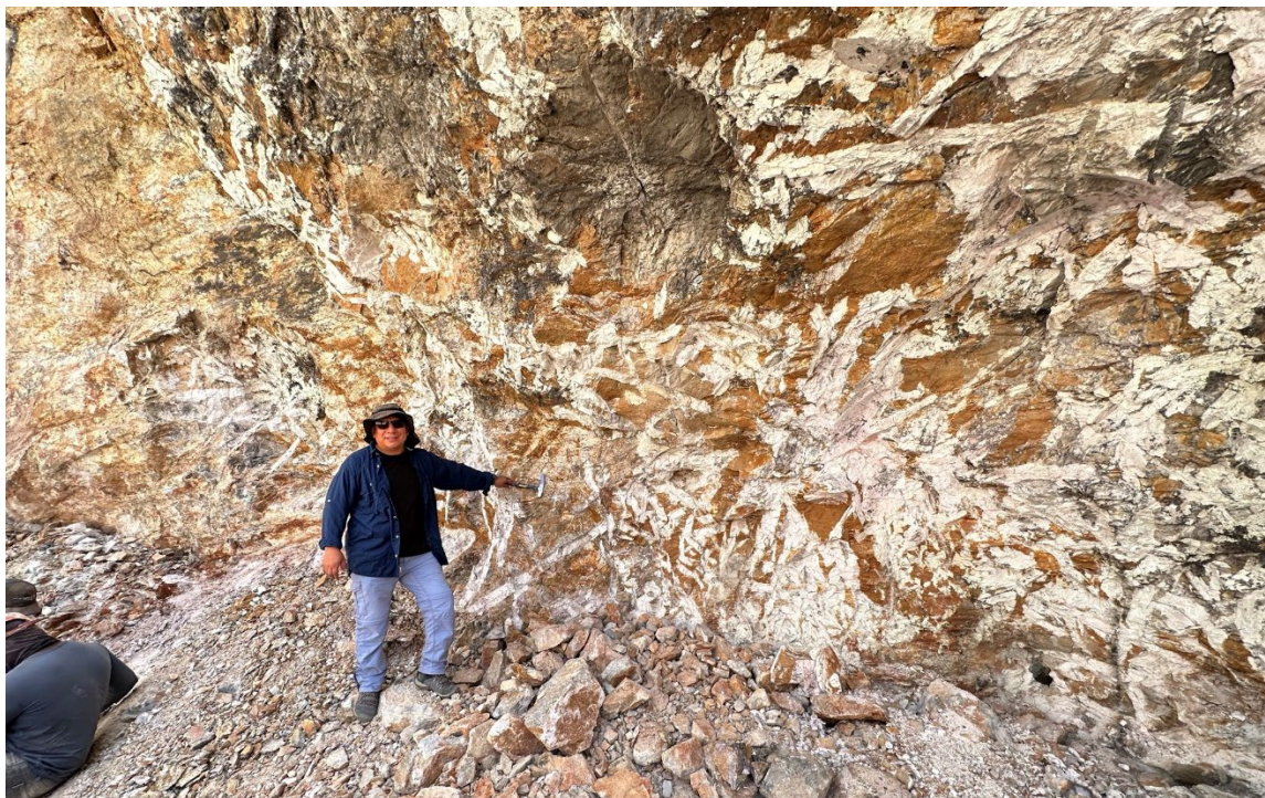
Figure 4: Solis geologist standing in the artisanal workings with large white spodumene crystals exposed in the face. Spodumene is a pyroxene mineral consisting of lithium aluminum inosilicate, \text{LiAl}(\text{SiO}_3)_2 , and is a commercially important source of lithium
