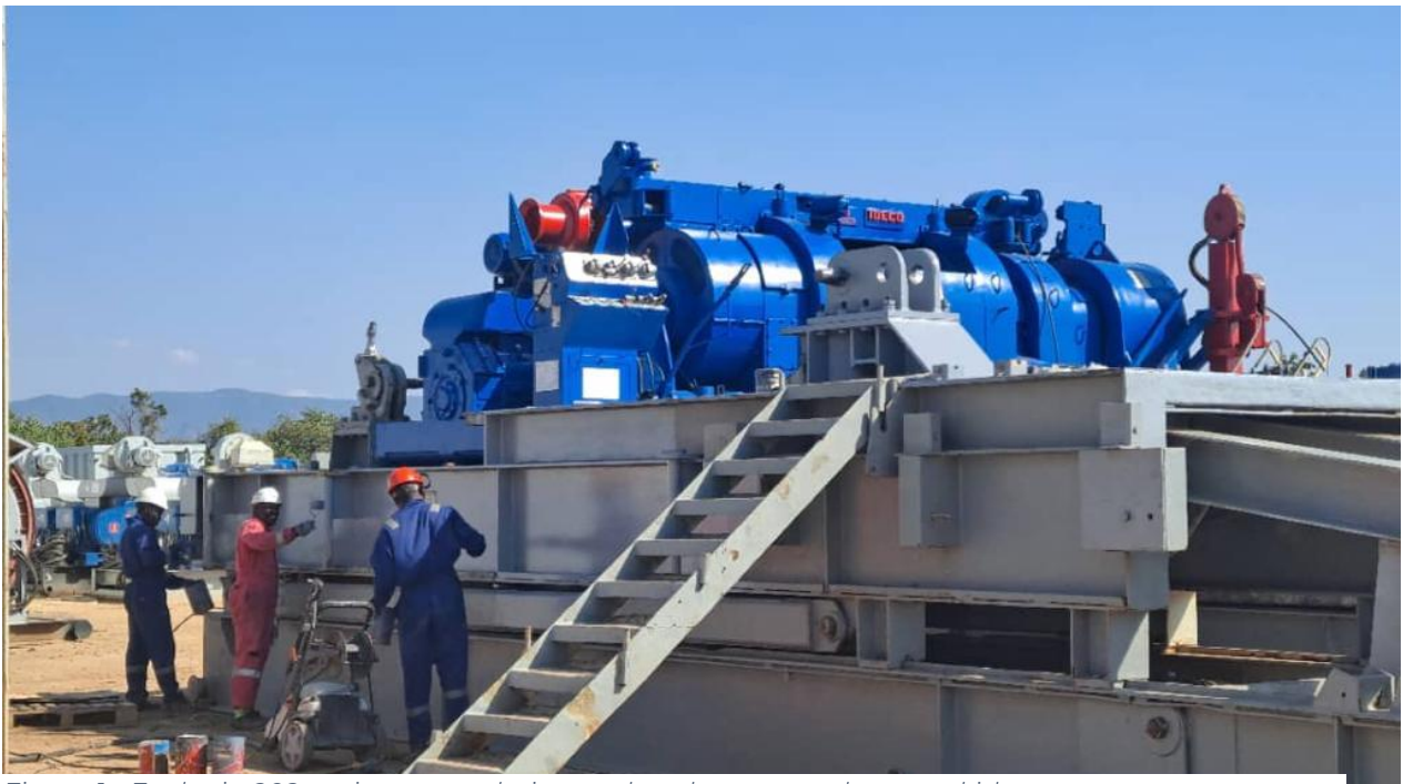
Figure 1 - Exalo rig 202 maintenance being undertaken on mud pump skid
