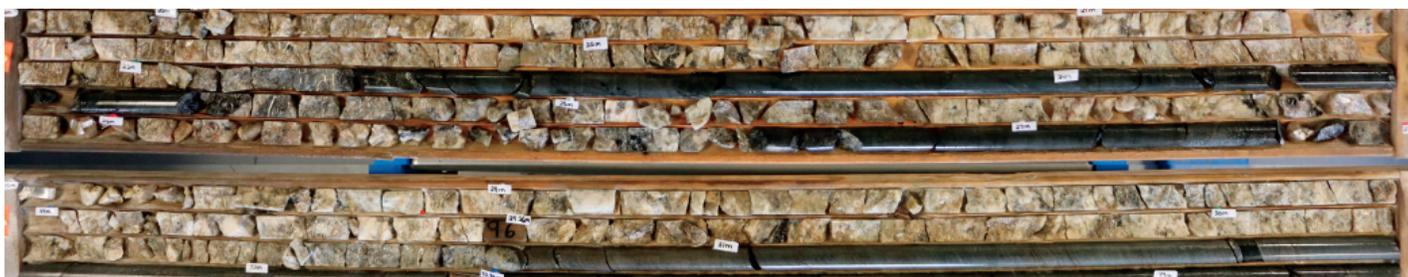
**Figure 1** Core XL-17 - 11.0m of unsampled spodumene bearing pegmatite from 19.8m.
