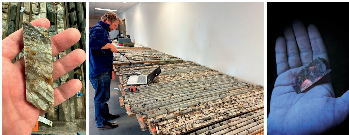
**Figure 2** Large grained Spodumene (left image), Chief Geologist (centre image) logging historic drill core, and Under UV light (right image) pegmatite with spodumene mineralisation within the core shows as pink fluorescence.
