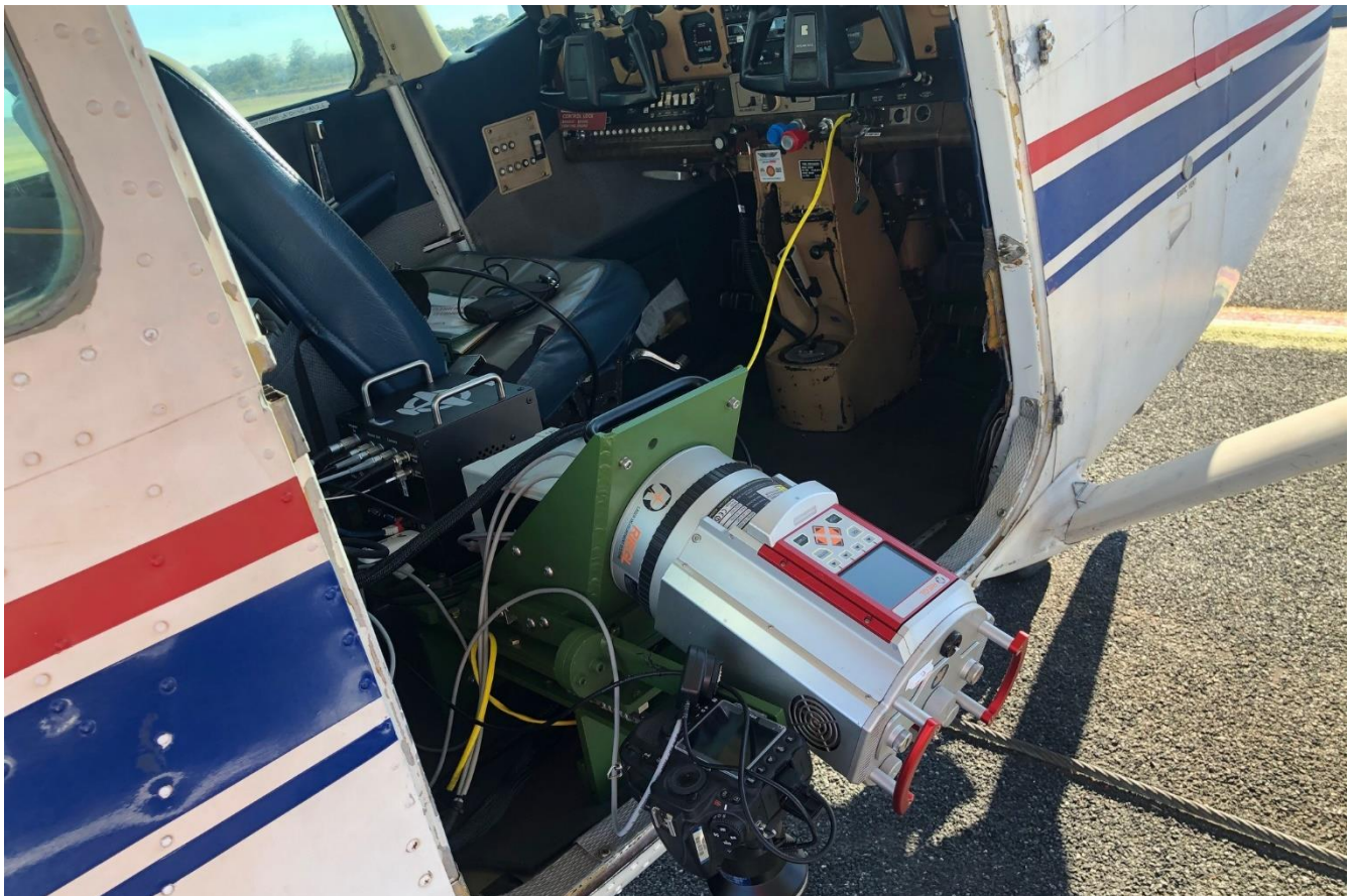
Figure 1: Airborne LiDAR system used for the survey.
