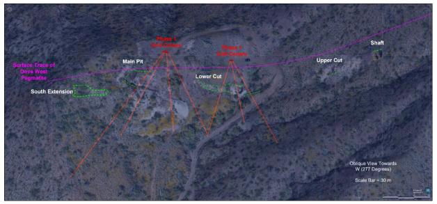
*Figure 2: Planned Phase 1 drill collars and hole traces targeting shallow subsurface extensions to the Dove West spodumene pegmatite exposed in the Main Pit and Lower Cut and along the South Extension of the historic Dove pegmatite mine.*
