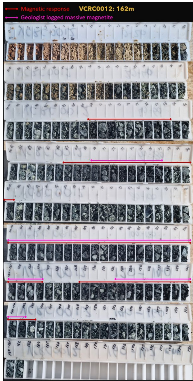
Figure 3; Drillhole chips from VCRC0012 showing the occurrence of highly magnetic material (red highlights) and zones of massive magnetite as logged by Viking geologists (pink highlights).
