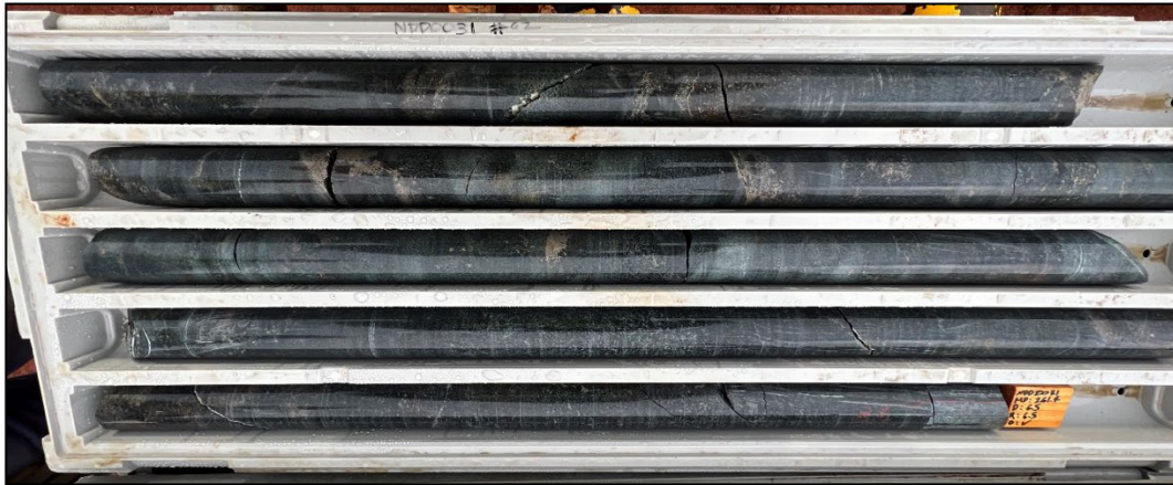
Figure 2: NDD0031 from ~258-261.4m with disseminated sulphides and clots.
