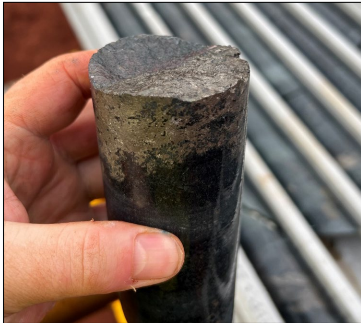
Figure 1: NDD0031 core ~257.7m of possible pentlandite, pXRF indicated 3.29%Ni and 0.28%Cu.
