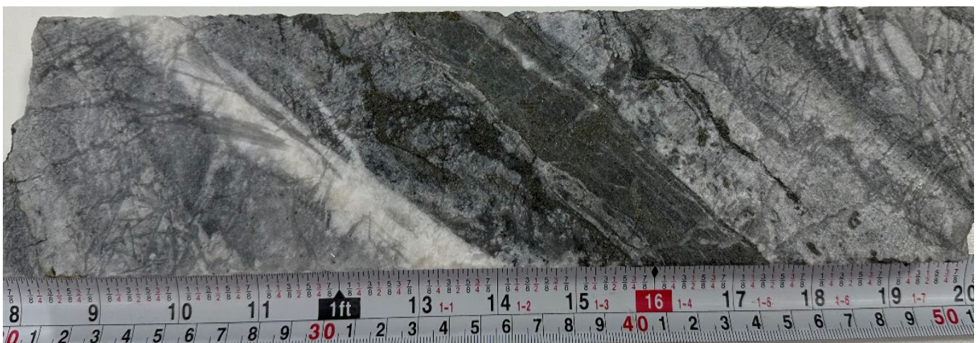
Plate 2: CVDD23-101- 404.6m. Massive epithermal quartz-gypsum-barite-carbonate-pyrite-arsenopyrite-sphalerite vein.
