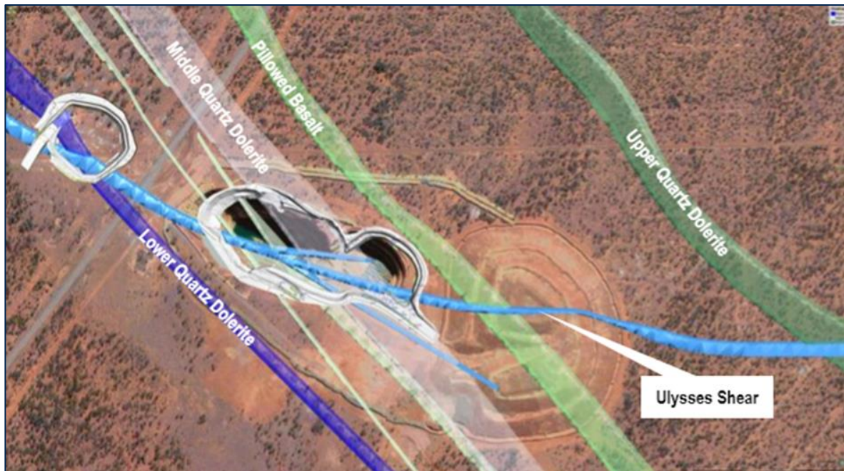
Figure 9: Aerial photo of Ulysses draped with the modelled geology projected to surface
