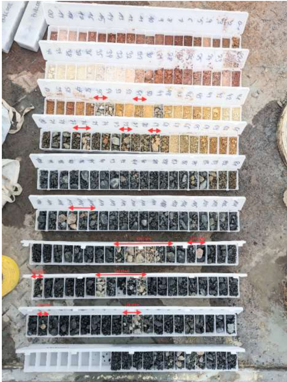
Figure 3: RC Drill Chips from TNRC001 0-192m showing Pegmatite Zones in red
