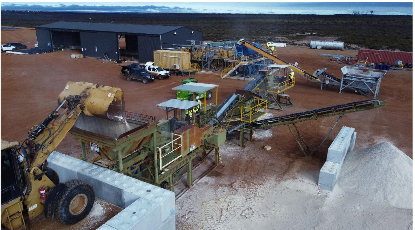
**Figure 1 – Hopper at Crushing Circuit being loaded at Kat Gap.**
