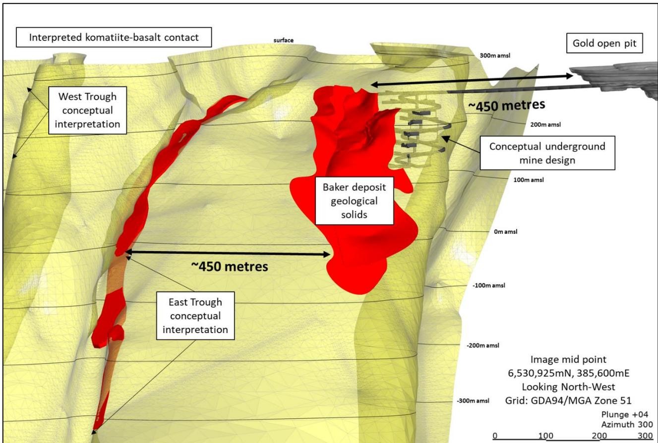
**Figure 1:** Perspective view looking (NW) from the komatiite hanging wall towards the basalt footwall illustrating spatial relationship between West & East Troughs (to the left) and Baker (right).
