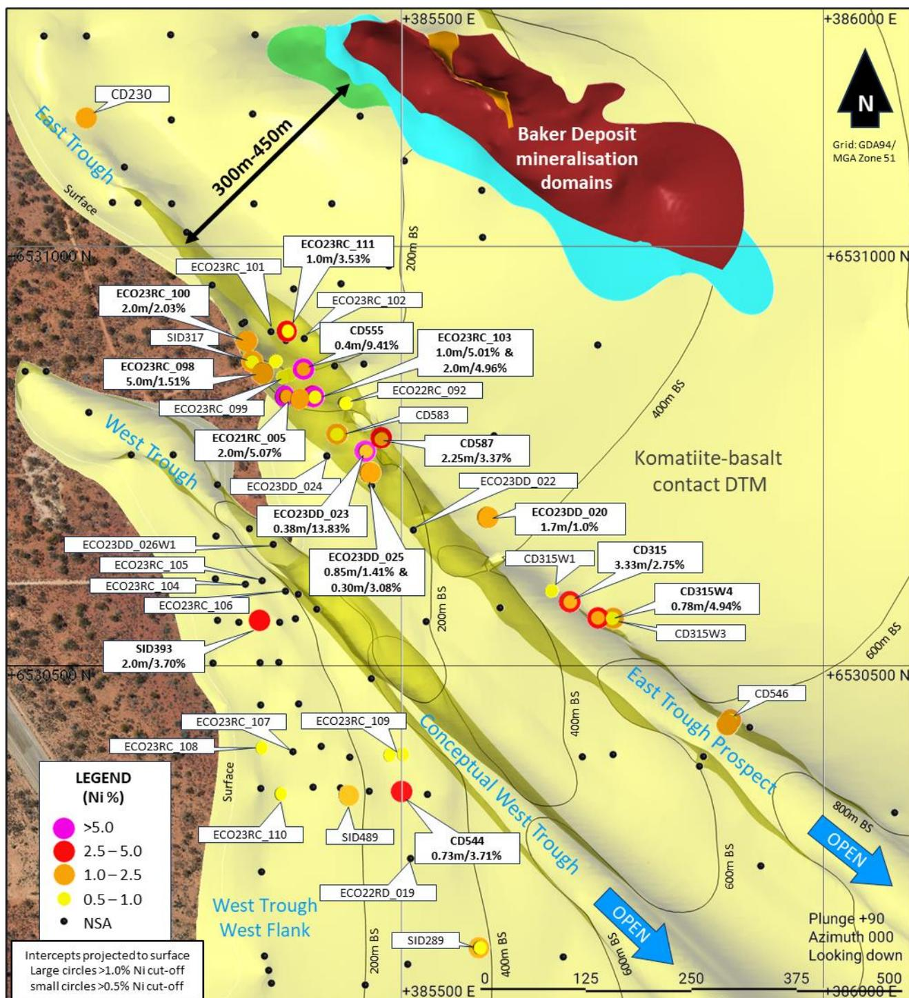
**Figure 2:** Plan view of East and West Trough targets highlighting recent results. The yellow wireframe Digital Terrain Model (DTM) surface is the interpreted komatiite-basalt contact with contours in metres below surface (m BS). Note: annotated drill holes without m/Ni % labels are reported in Annexure 2a and 2b and omitted for ease of viewing.
