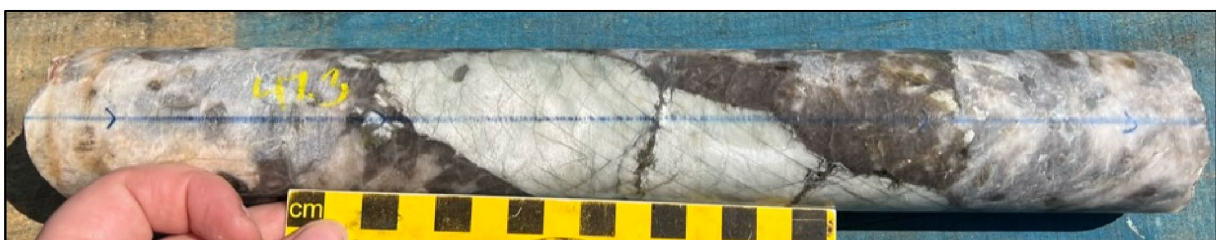
Figure 2 - Core showing coarse grained spodumene mineralisation in hole 23FL-005
