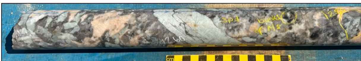
Figure 3 - Core showing coarse grained spodumene mineralisation in hole 23FL-007
