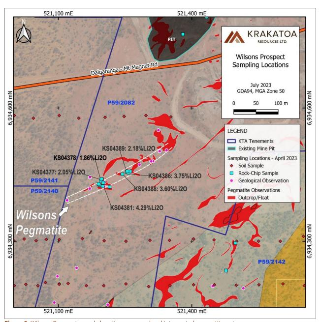
**Figure 3:** Wilsons Prospect sample locations, mapped and interpreted pegmatite outcrops.
