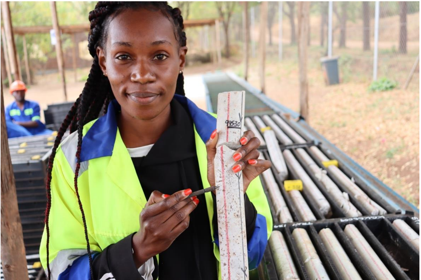
Image 2: Serah Misuku, Site Program Geologist, with a section of drill core showing textural features of monazite, strontianite and baryte (replacing original burbankite crystal pseudomorphs) at 995.3m downhole. Estimation of abundance of monazite range 0.5% to 3% in a 0.5m interval at 995.3 to 995.8m consistent with the range of observations for the entire drill hole from surface to 999.77m.
