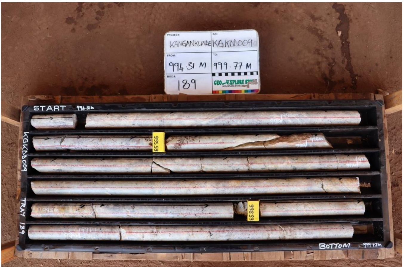
Image 1: Pieces of the drill core from KGKRC009 that appear to show the crystal texture of the monazite at depth, similar to the textural consistency of mineralisation observed at surface. Estimation of abundance of monazite range 0.5% to 3% 2 for this interval from 994.3m to 999.77m consistent with the observation in entire hole.
