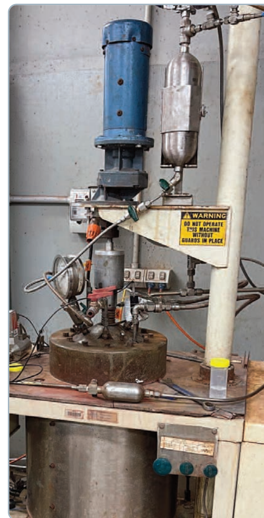
Ardea's Goethite ore undergoes batch high pressure acid leach autoclave test work
