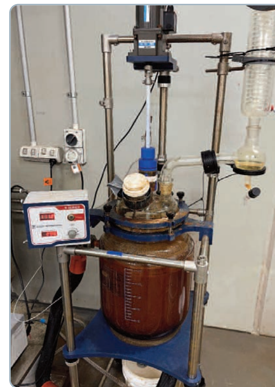
Ardea's Saprolite ore undergoes batch atmospheric leach test work
