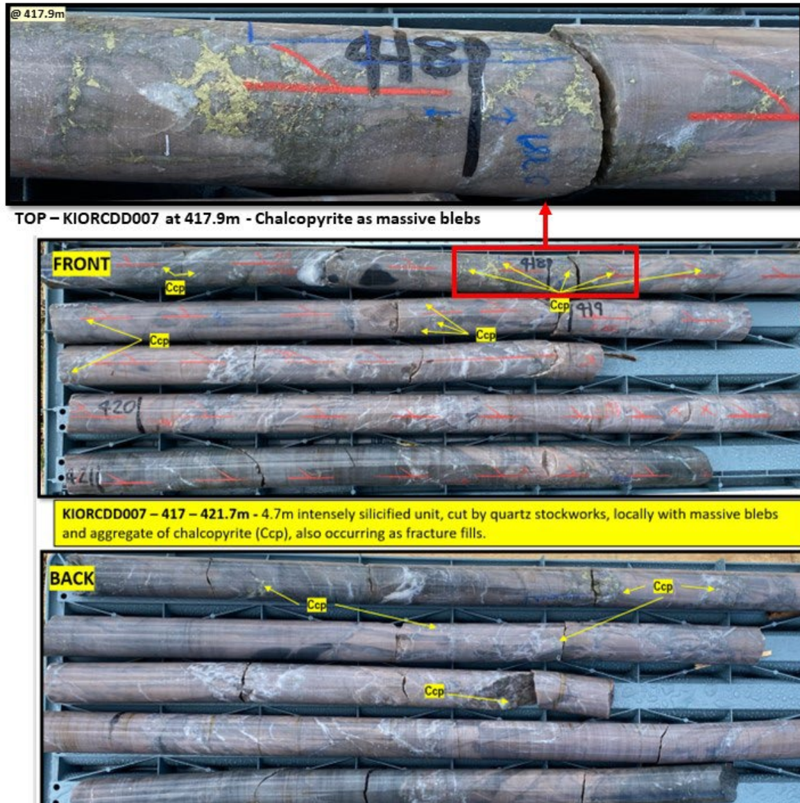
Figure 5: Drill hole KIORCDD007 – Intensely silicified meta sediment cut by quartz stockwork veins containing chalcopyrite as fracture fill and blebs.
