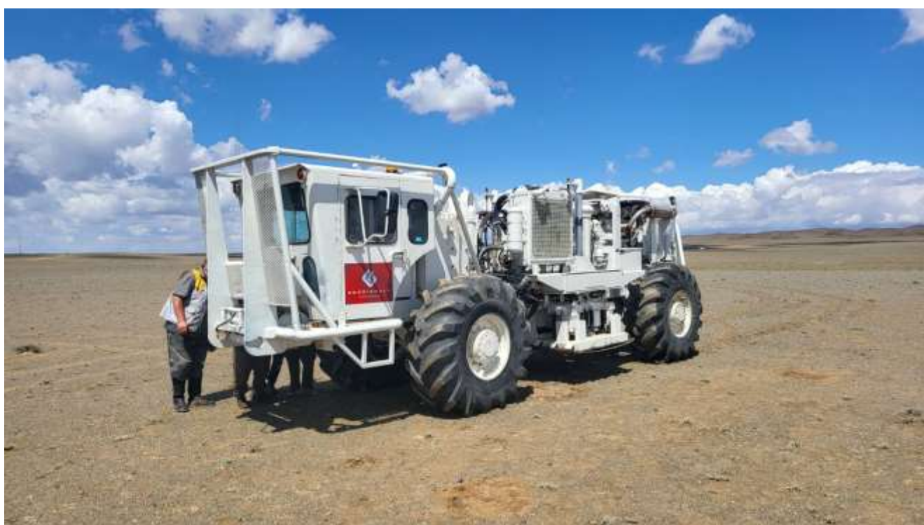
Figure 1 – Vibroseis truck at TTCBM Project location showing ease of land access for the crew.
