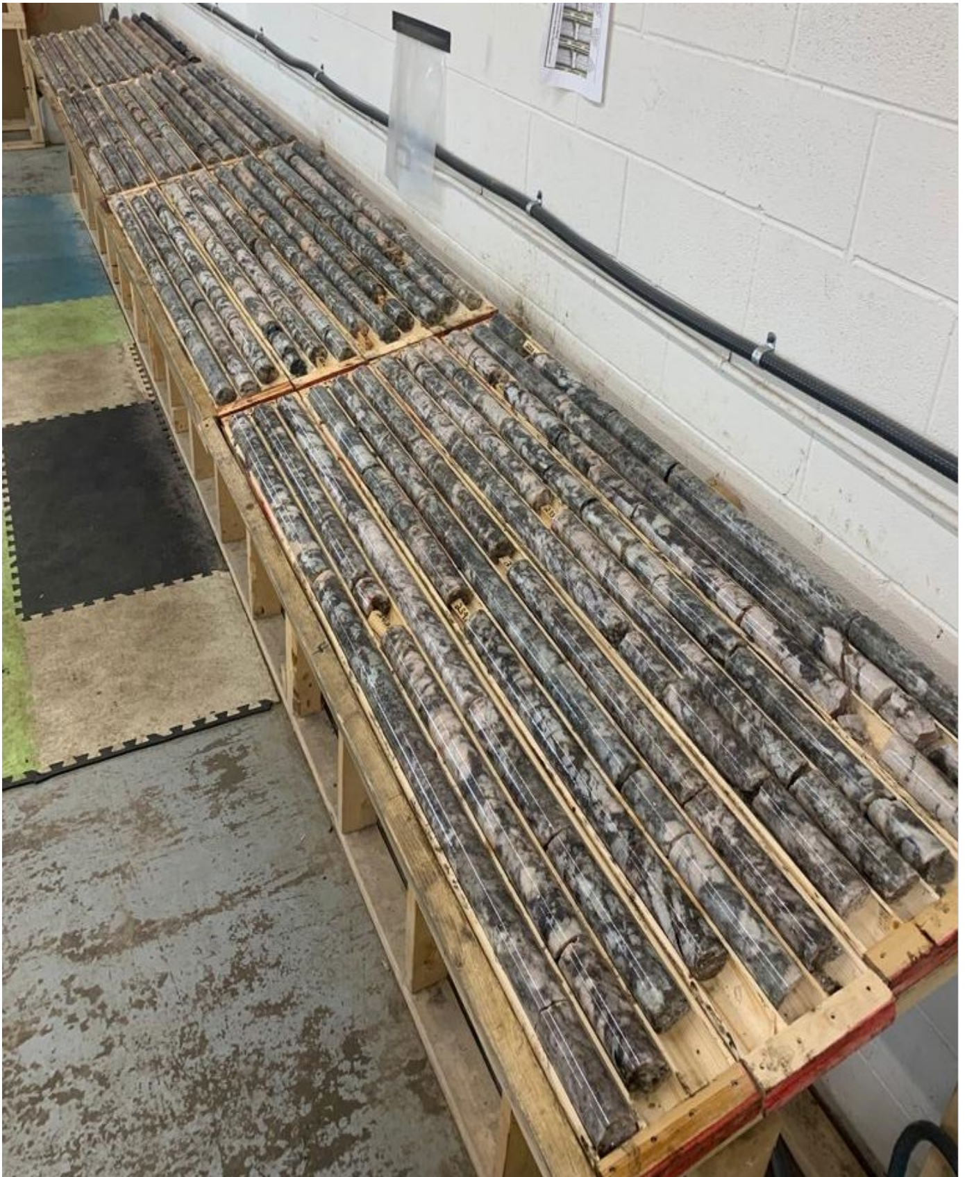
Figure 1 – Approximately 74.4m of continuous spodumene mineralisation from drill hole MF23-207, intercepted from 176.15m to 250.55m down-hole
