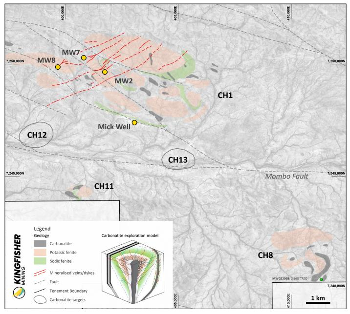
Figure 1: CH1, CH8 and CH11 carbonatite intrusion centres and associated REE mineralisation. The Mombo Fault and newly identified CH12 and CH13 carbonatite targets are also shown. The carbonatite exploration model is explained on page 7 of this announcement.
