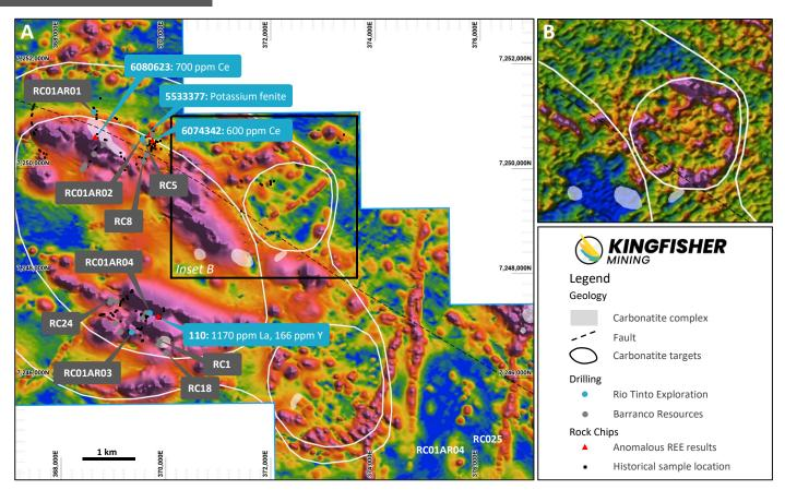
*Figure 4:* Total magnetic intensity (A) and thorium responses (B) showing compelling carbonatite targets. Drill hole locations (grey boxes) described in Table 1 and surface sample (blue boxes) are also shown.
