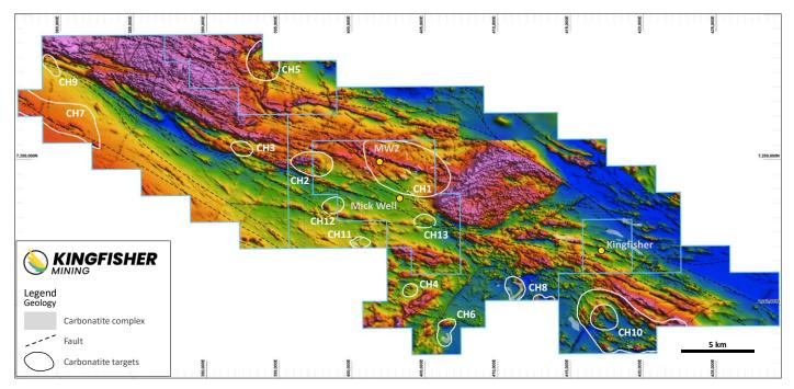
**Figure 2:** Total magnetic intensity for the 54km Chalba target corridor showing priority carbonatite targets and interpreted faults. Targets are labelled CHI to CHI0 and were selected based on the magnetic, thorium and potassium responses from the airborne geophysics surveys.
