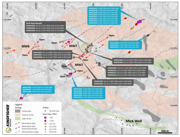
**Figure 3:** Mick Well mineralisation and rock chip results (blue boxes). Drill results are shown in grey boxes (see ASX:KFM 7 February 2023, 5 July 2022 and 24 March 2022). Results are stated as Total Rare Earth Oxides (TREO%) and total  $Nd_2O_3 + Pr_6O_1$  (%) content.
