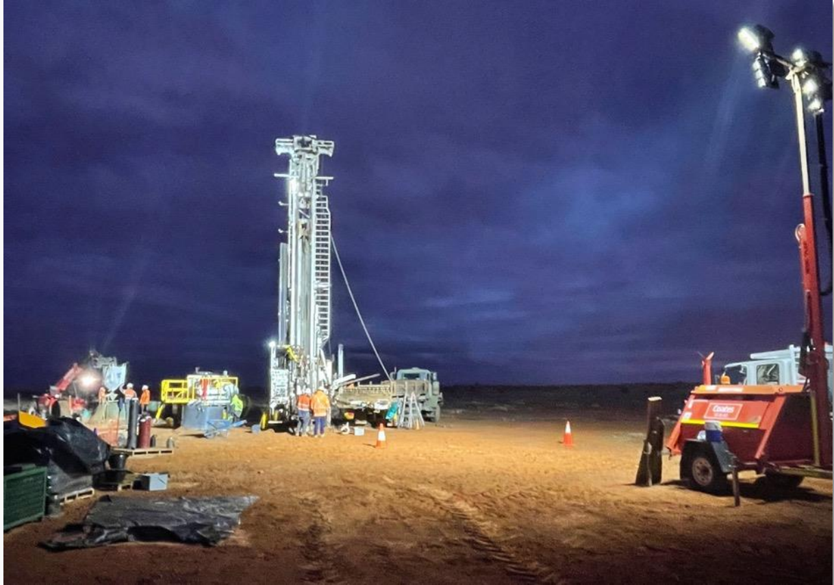
Figure 5. MJ Drilling Rig (UDR1200) onsite - Drill Hole ID 23PK02 - Target RH02, TD 622m.
