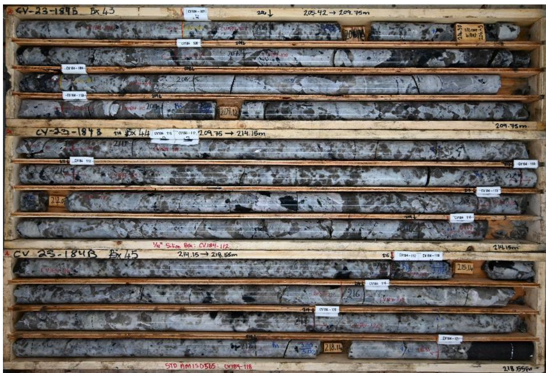
Figure 6: High-grade (~1.9% \text{Li}_2\text{O} ) spodumene pegmatite in drill hole CV23-184, the most westwardly drill hole completed to date at CV5.
