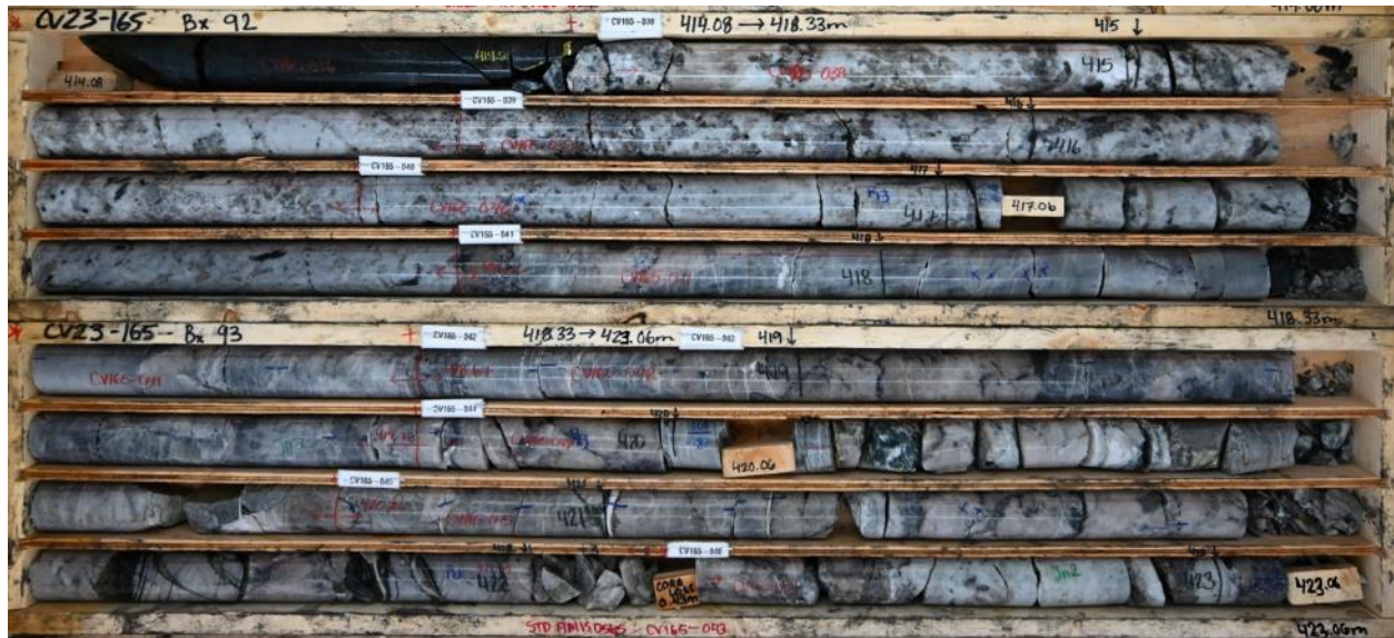
Figure 7: High-grade (+2.0% Li 2 O) spodumene pegmatite in drill hole CV23-165, including intersection of 2.2 m at 5.02% Li 2 O (417.6 m to 419.8 m), one of the most eastwardly drill holes completed to date at CV5.
