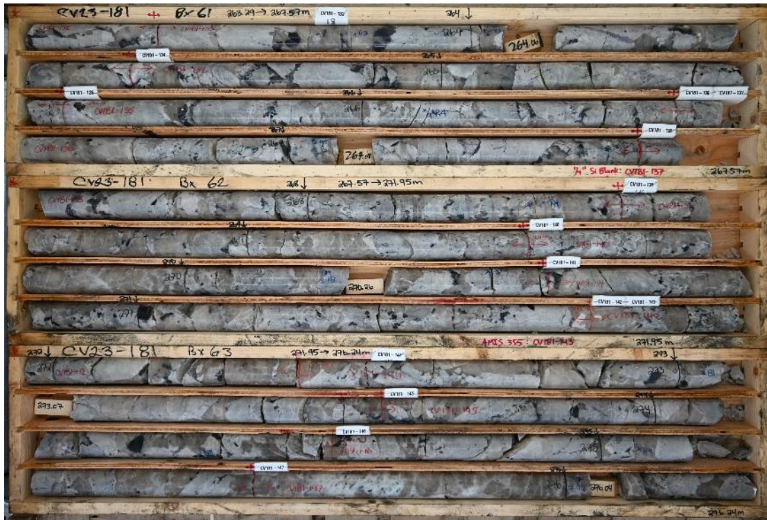
Figure 5: High-grade (4+% \text{Li}_2\text{O} ) spodumene pegmatite from the Nova Zone in drill hole CV23-181.
