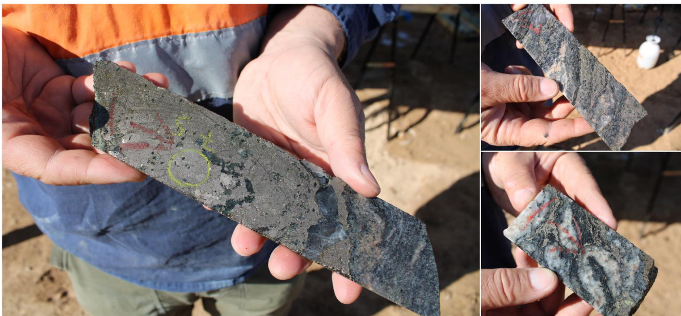
Figure 2: W21 prospect - WL23-370 Stringer Sulphides from 400m including a 30cm zone of semi massive sulphides - left (90% pyrrhotite, 10% pentlandite).
