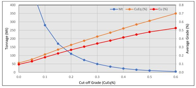
Figure 3. Indicative grade-tonnage curve for the Corvette and Kingswood deposits.
