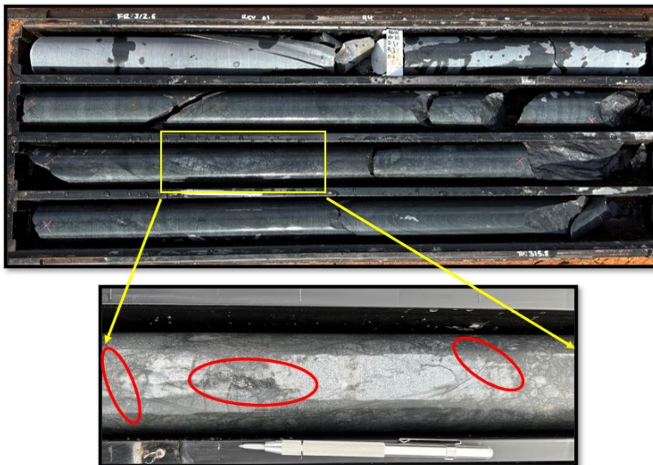
Figure 4: An example of mafic breccia with chlorite-epidote alteration and disseminated pyrrhotite/pyrite mineralisation (Rev-01, 313.5 to 315.8m)
