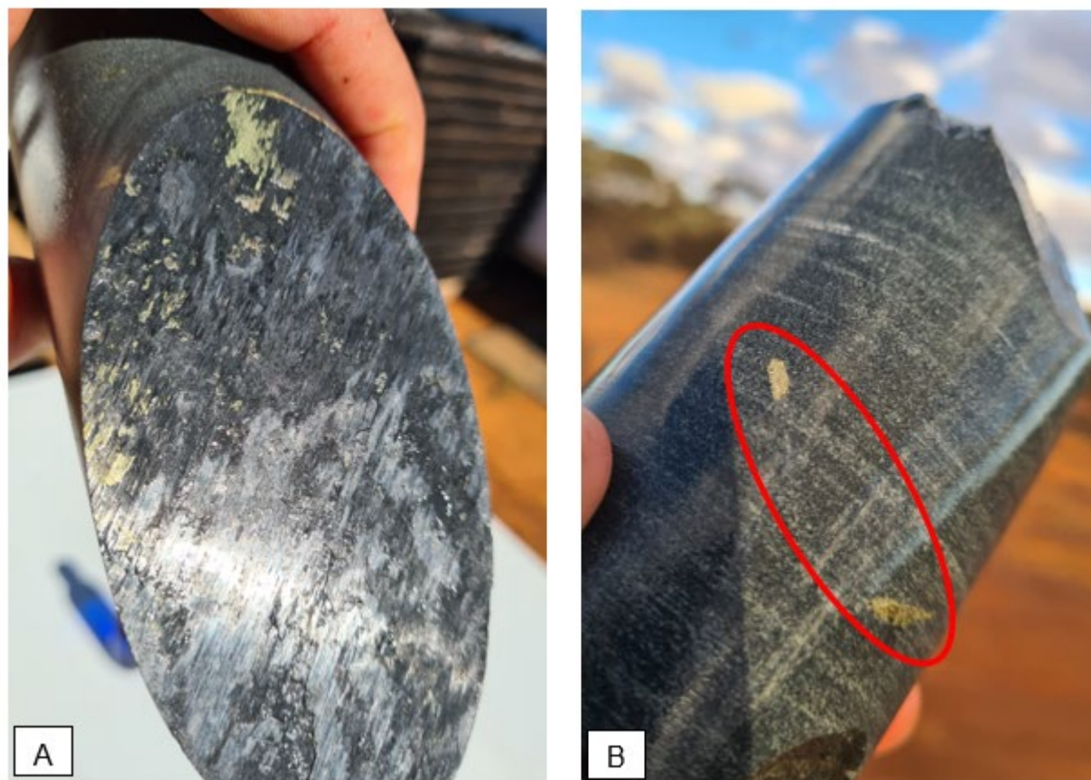
Figure 5: Significant mineralisation in REV-05 core, A: disseminated chalcopyrite and sphalerite (314.9m, 5.7% Cu and 4.2% Zn, B: chalcopyrite (280.8m, 1.9% Cu)
