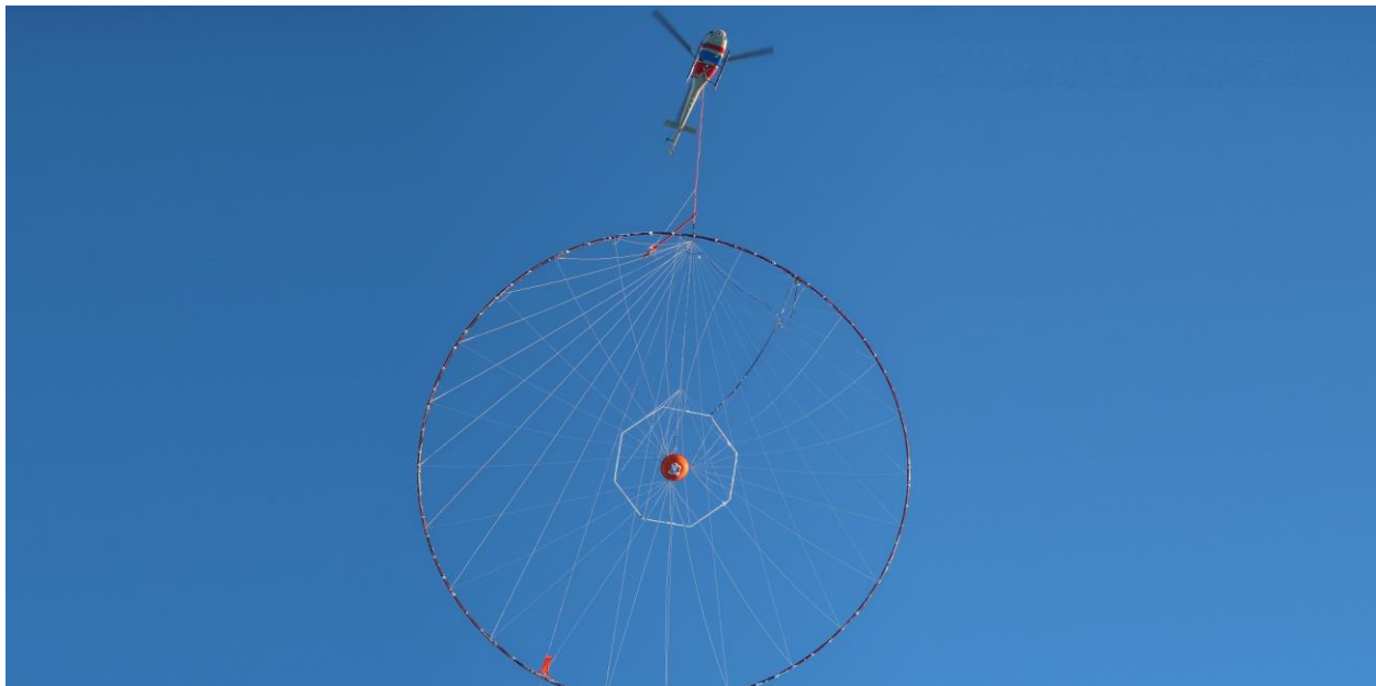
Figure 1: TargetEM Loop being tested
