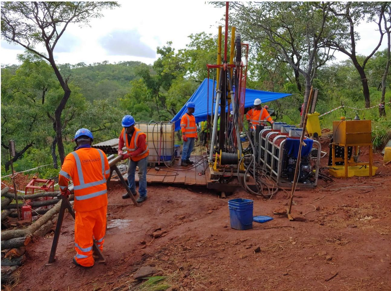
**Photo 1. Diamond drilling to test the subsurface geology and geochemistry beneath a high-grade haematite outcrop at the Kowouleni target where a rock chip sample collected returned an assay in excess of 64% Fe.**
