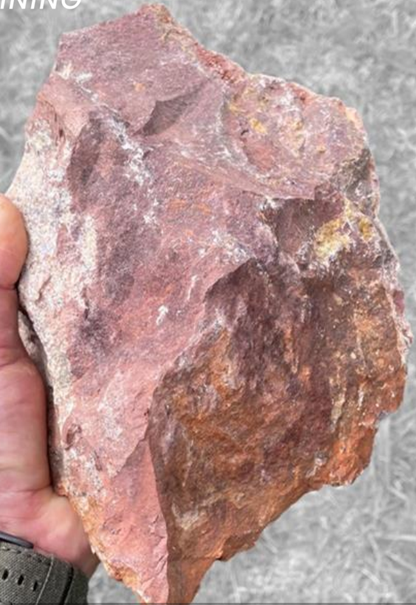
Image: Rock chip from MW2 with >40% TREO and 6.5% NdPr
