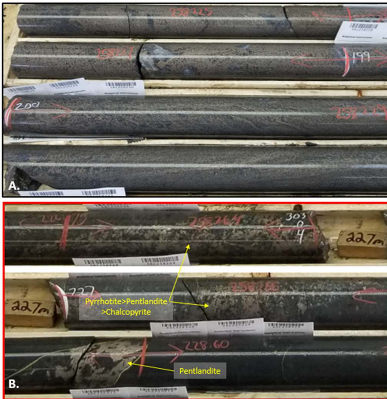
Figure 3 – FLC-2023-057 core photos. A. “Sulphide Zone”. B. “Nickeliferous centre of mela-gabbro intrusion”. Hole depths marked on core in white. Refer to Table 1 for descriptions of the core.
