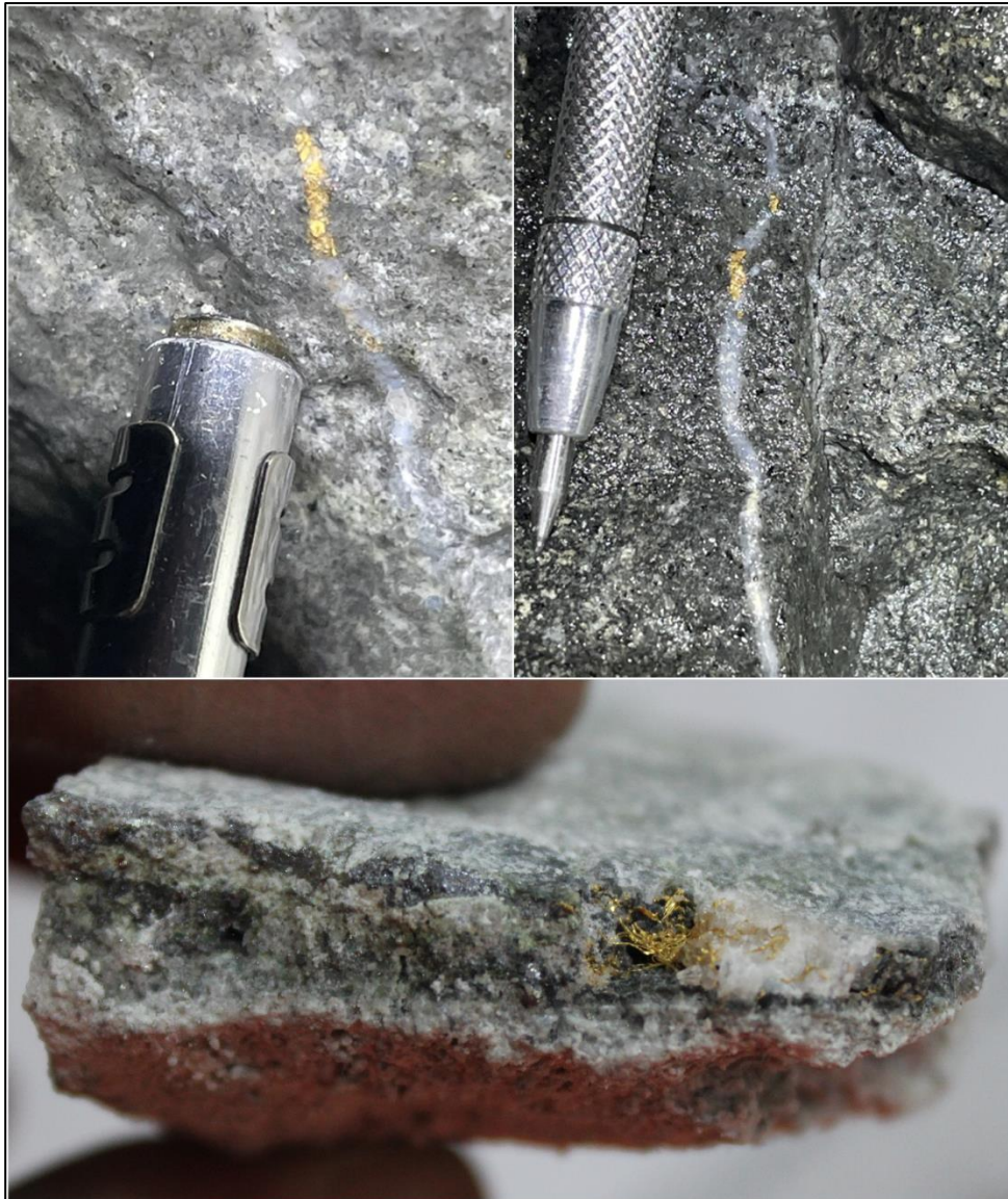
Figure 4. Examples of visible gold identified during sampling. Scratcher pen used for scale in top two images. Width of sampled in bottom image is 4.5 cm.
