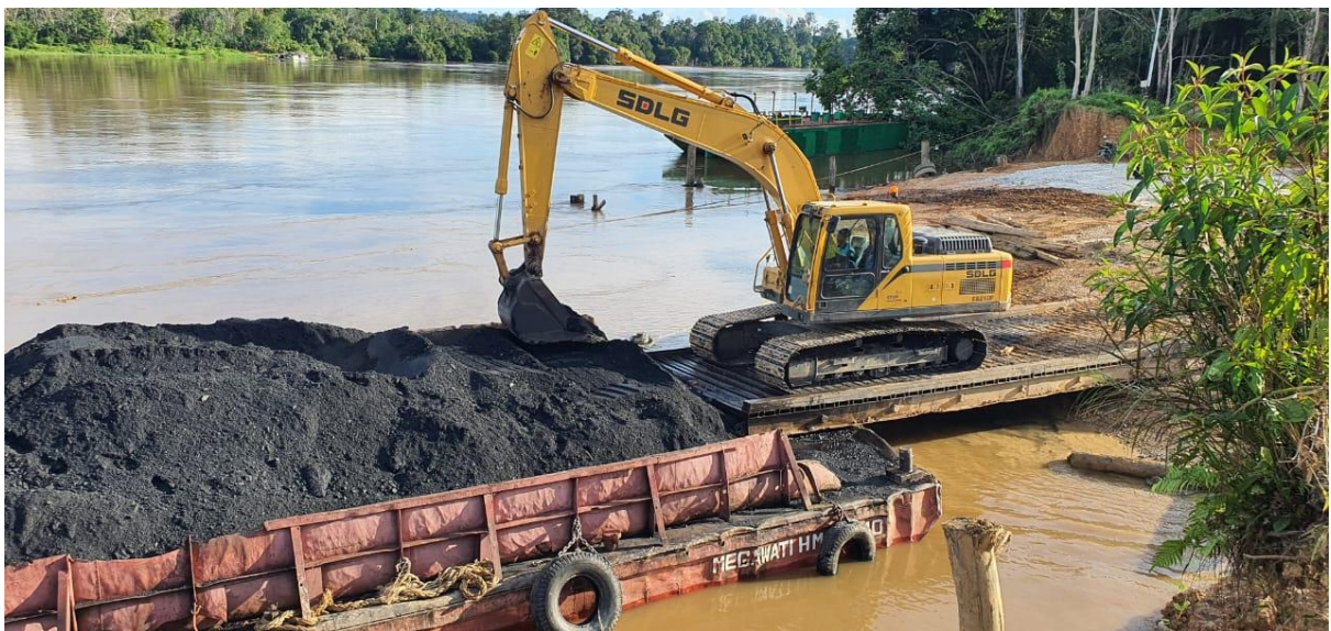
Coal loading onto barges at the Krajan Jetty
