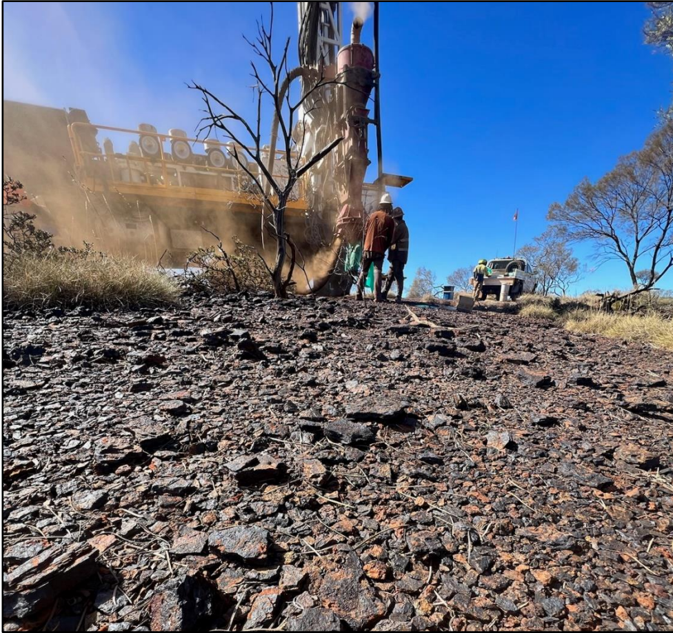
Figure 2. RC drill rig drilling on the KR1 target overlying outcropping manganese enriched shale within recently acquired license E46/1383
