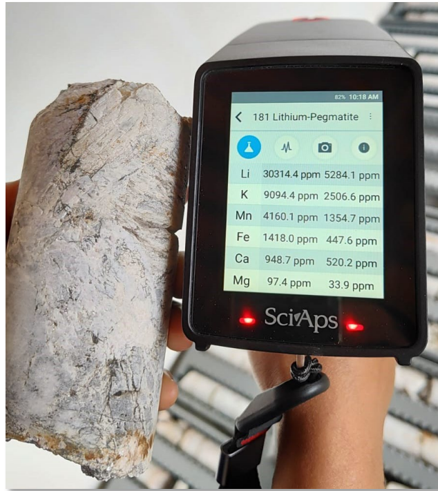
Figure 2: SciAps LIBS (Laser induced breakdown spectroscopy) handheld analyser reading on spodumene within core sample interval 44.3m in hole JADDH00003#.
