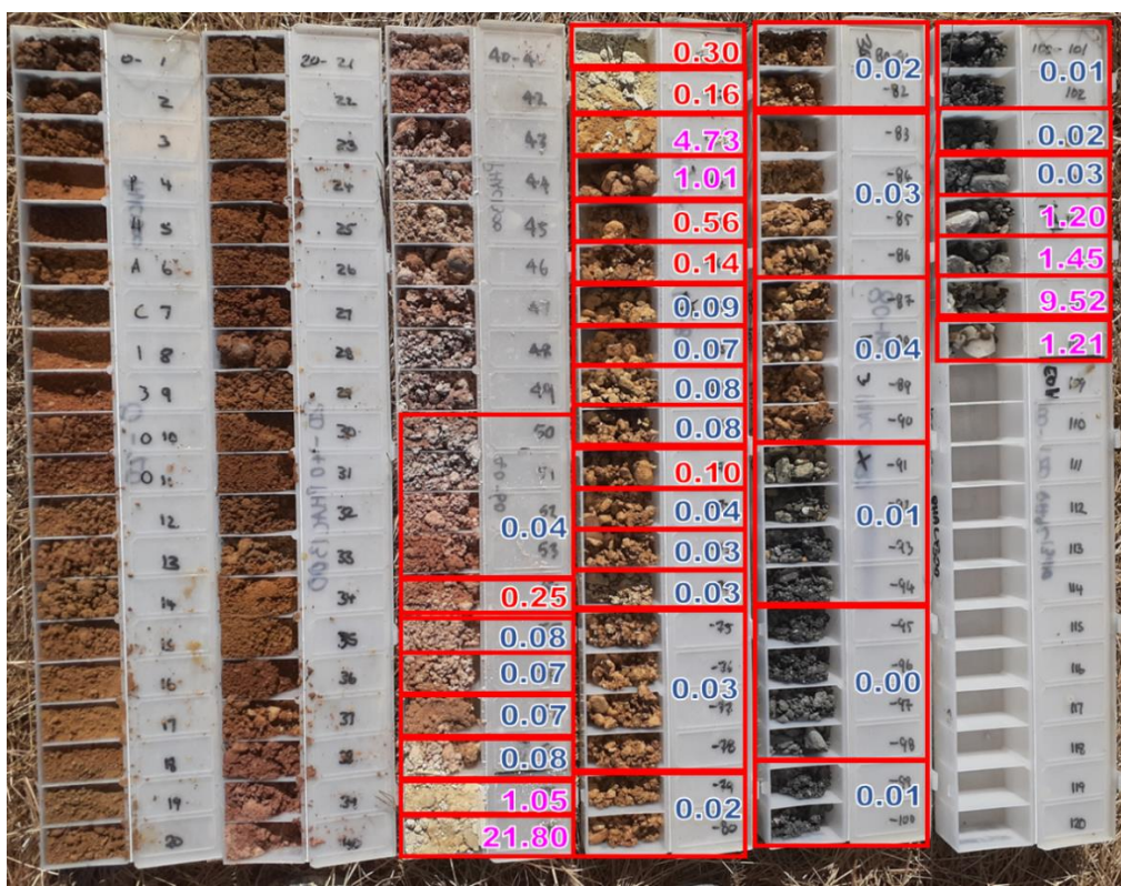
Figure 5 Chip tray photo of hole PHAC1300 showing the high-grade zones (g/t Au) in the saprolite, and in primary mineralisation at the base of the hole
