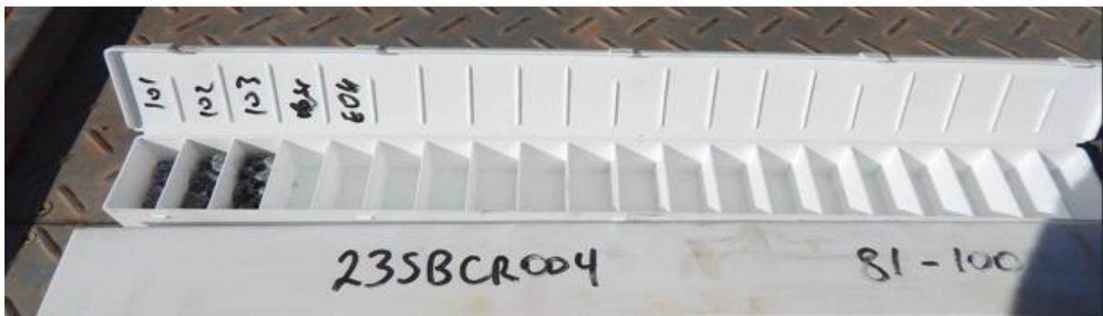
**Picture 3.** Chip tray showing 1m RC drilling samples, each box is representative of a ~1 meter interval in hole 235BRC004 from the Smokebush pegmatite drilling campaign, refer to above caution note.
