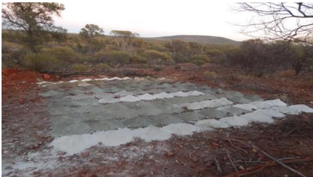
**Picture 4.** Drill spoil material from hole 235BRC002 showing multiple intervals dominated by quartz and feldspar characterised by their light grey to white colour and logged as pegmatite.
